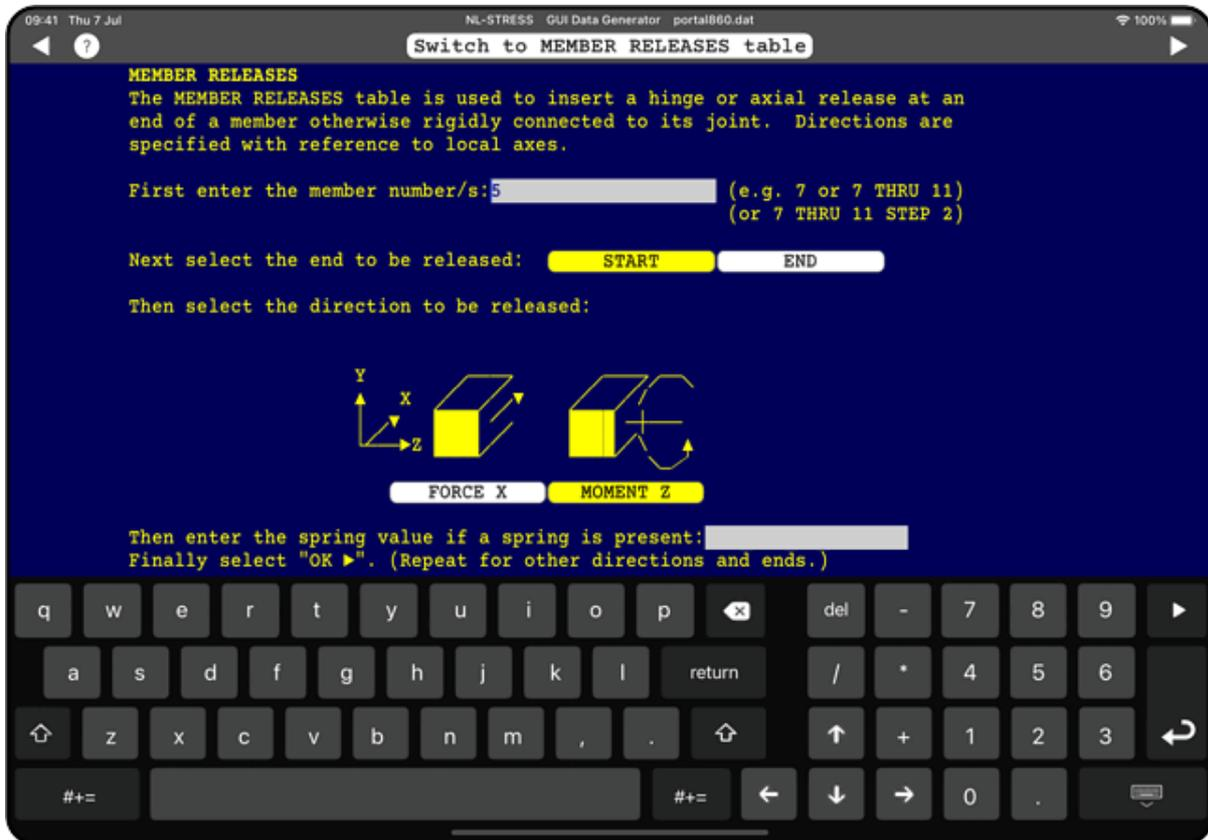
Figure 5.35: GUI MEMBER RELEASES entry for PLANE FRAME.
