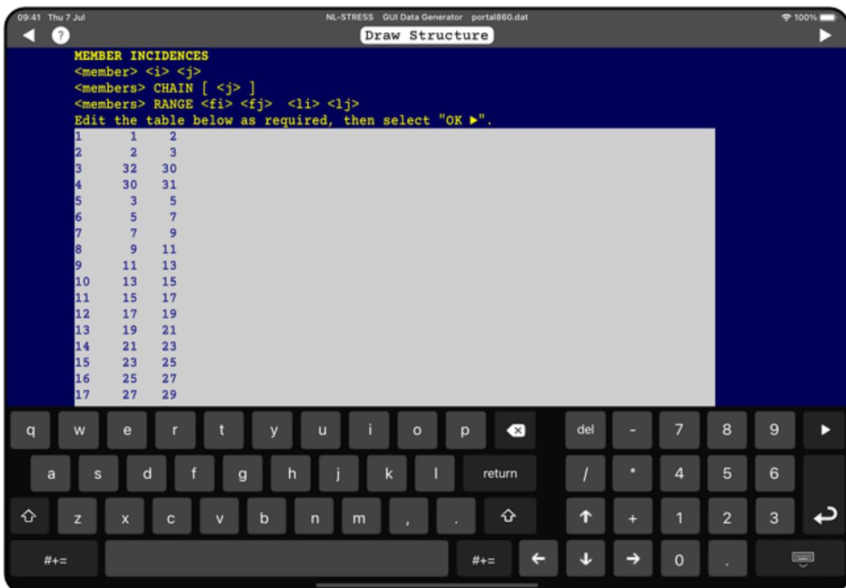
Figure 5.33: GUI MEMBER INCIDENCES table after Draw Structure.
