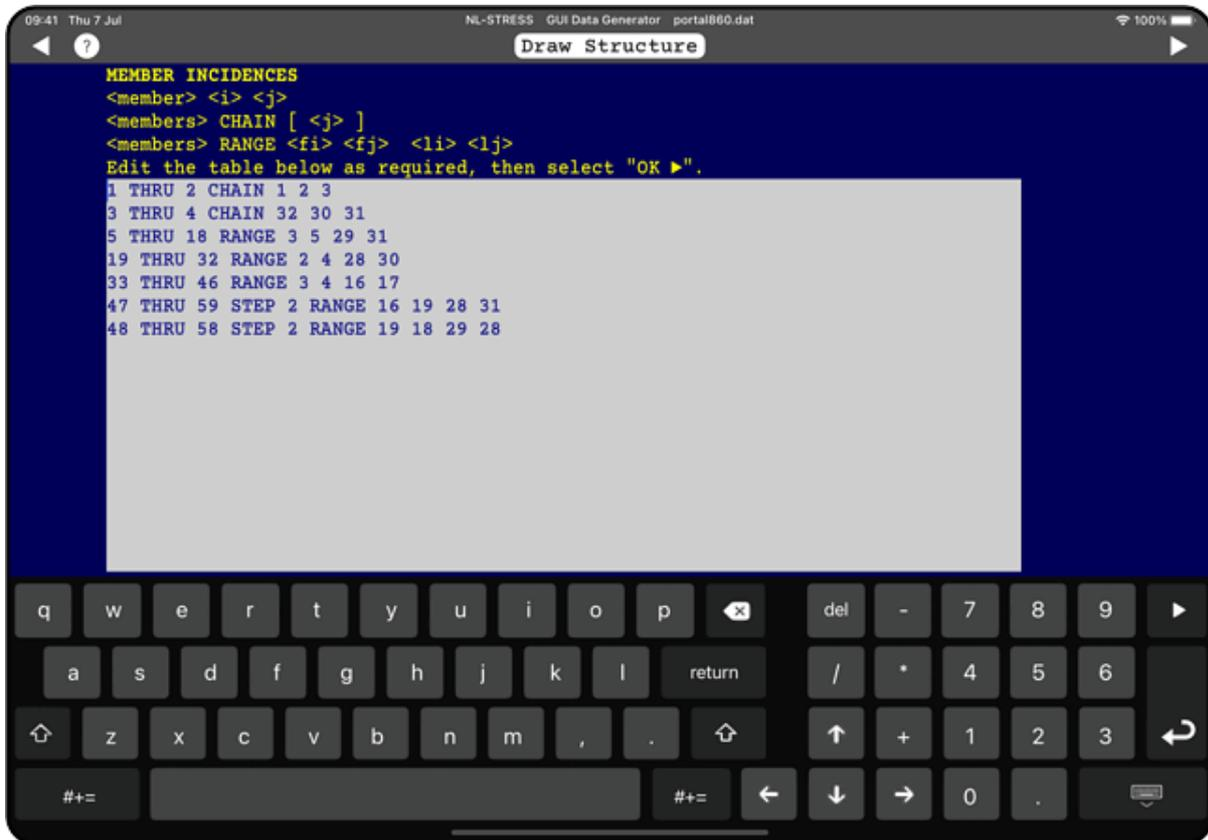
Figure 5.32: GUI MEMBER INCIDENCES table.
