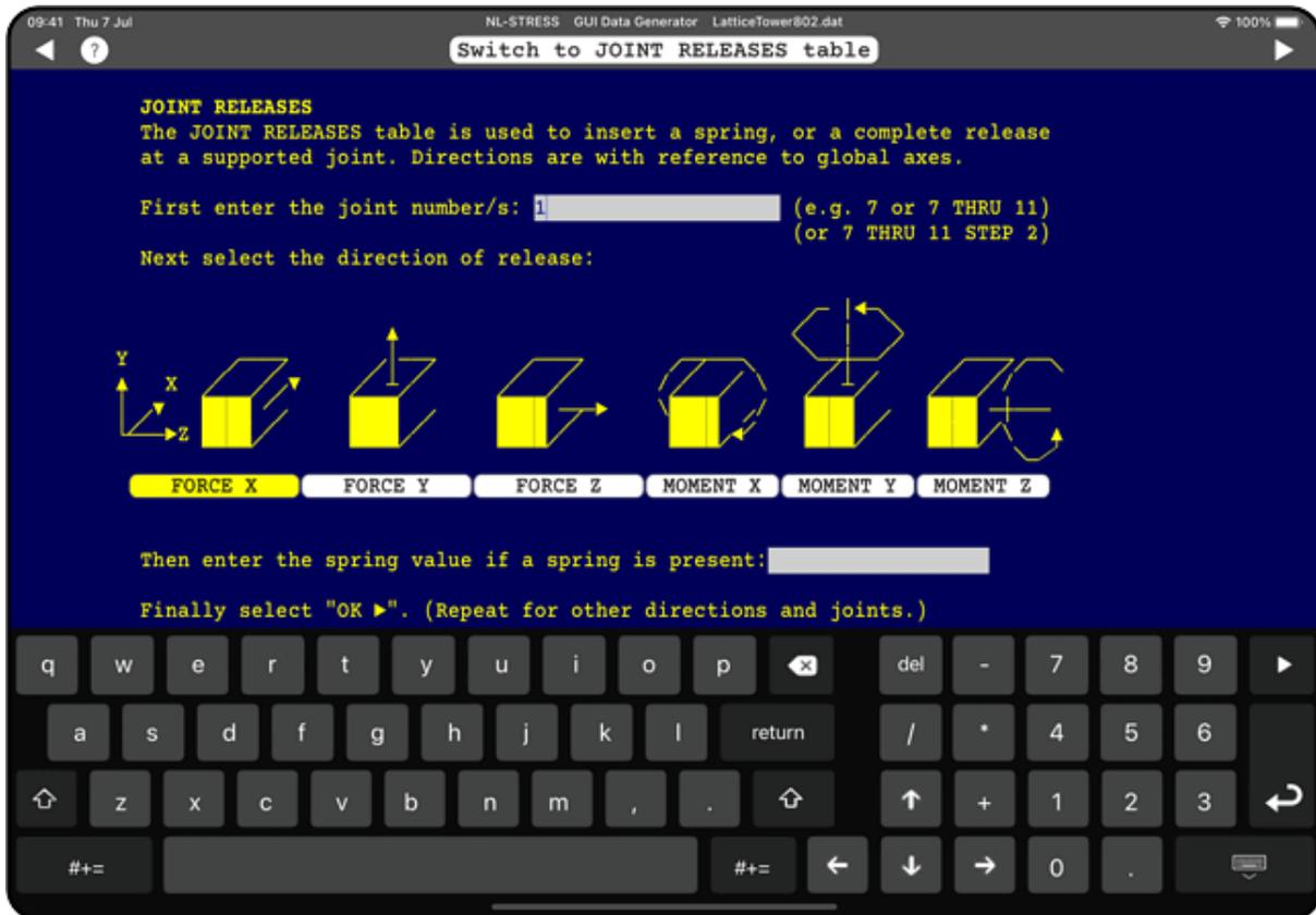
Figure 5.29: GUI JOINT RELEASES entry for SPACE FRAME.
