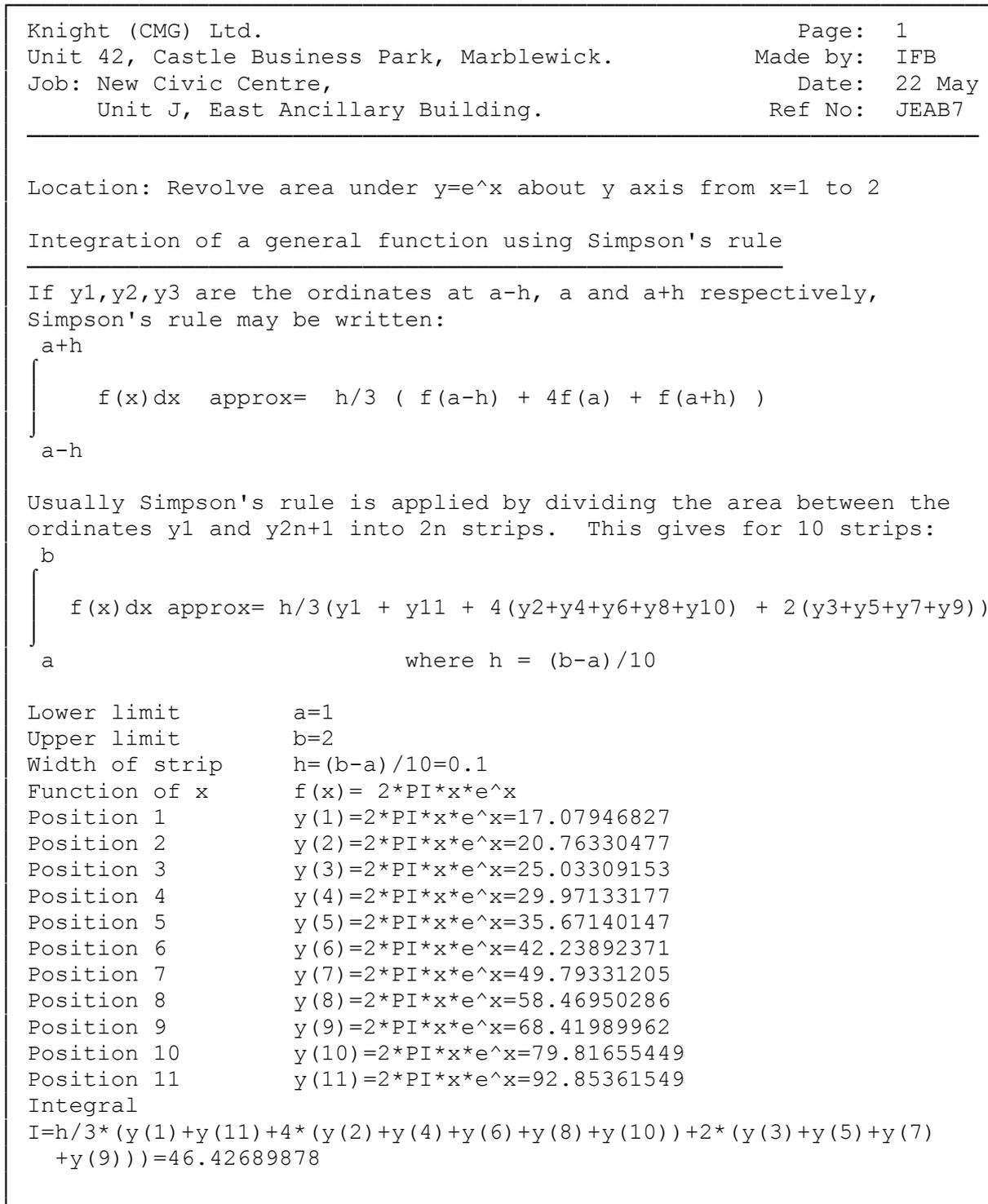
Figure 1.1 Typical calculation produced by SCALE
