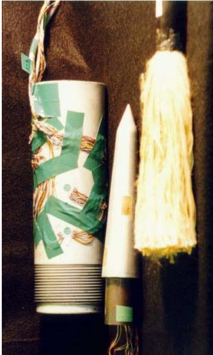
Figure 7.1: Strain gauging of a 60 tonne Parafil spike and barrel. Six rosettes were placed around the outside of the barrel, four in the middle and two near the base. Four rosettes were placed in cavities on the surface of the spike, at the base, at the nose, and two in the middle; the connector used to pull the spike out after the test without damaging the wires can be seen.
