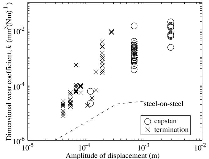
Figure 14: Effect of amplitude on dimensional wear coefficient.
