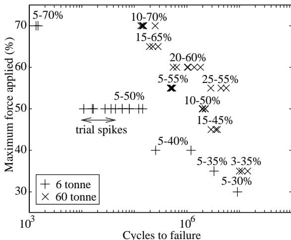
Figure 11: The lifetimes of 6 and 60 tonne Parafil G ropes subjected to cyclic loading.
