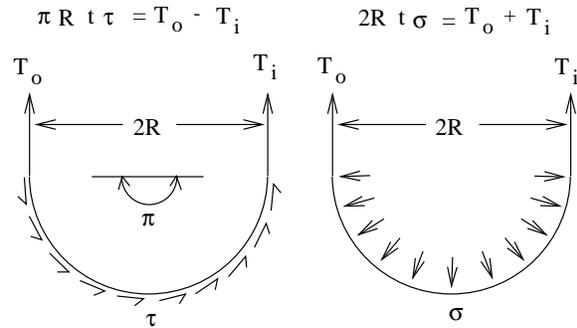
Figure 6: Estimation of average contact and frictional stresses on a capstan.
