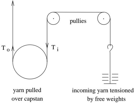
Figure 4: Apparatus used to measure yarn on solid friction.
