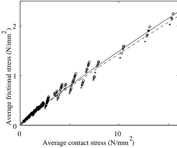
Figure 8: Visualisation of the average frictional stress versus average contact stress.
