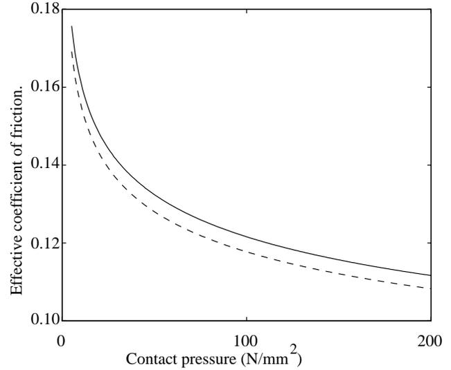
Figure 9: Equivalent Amontons' coefficients of friction ( $\mu = \tau/\sigma$ ) for Kevlar 49-on-aluminium.
