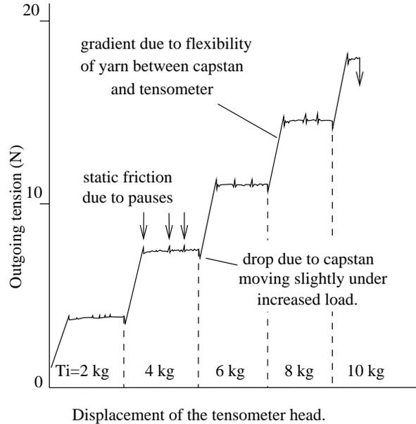
Figure 5: Plot of the outgoing tension for Kevlar 49 pulled over a 30mm aluminium capstan at 0.17mm/s.
