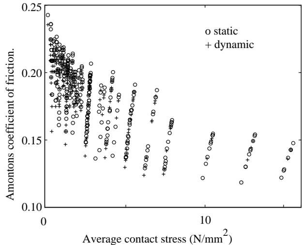
Figure 7: Effective Amontons' coefficient of friction,  $\mu$ , for Kevlar 49-on-aluminium assuming  $\mu$  is constant.
