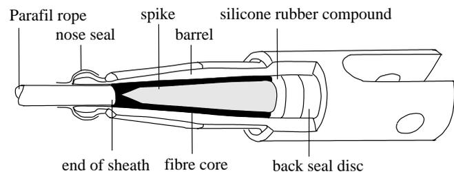
Figure 1: Spike and barrel Parafil termination.
