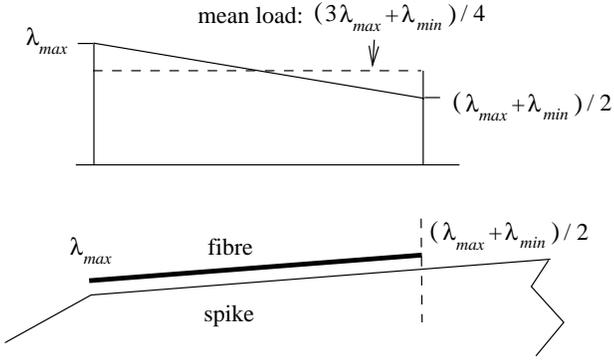
Load in fibres when unloaded:
