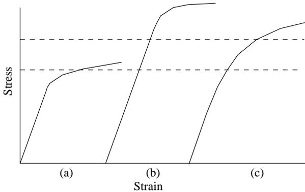
Figure 2: Stress-strain curves for various hypothetical asperity models.
