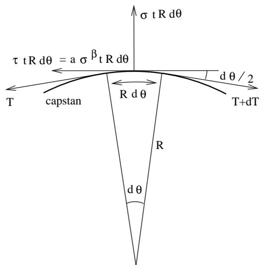
Figure 3: Forces acting on a segment of yarn running over a capstan.
