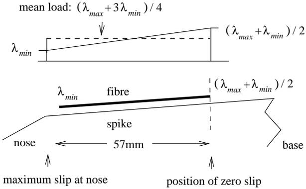
Figure 12: Schematic of the idealised load variation within a termination.
