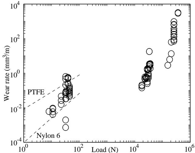
Figure 13: Effect of normal load on wear rate.
